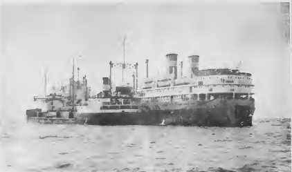
IT UNDECKED together like a mother whale and her nursing calf, the S. S. Cumaré reverses the rules here as she pumps 10,000 barrels of fuel oil aboard the "Southern Venture ," a British whale "factory." The lake tanker "topped off" the whaler outside San Nicolas harbor to save the ship's having to negotiate the entrance fully-loaded.
